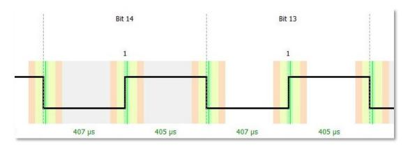
After reducing tx\_high\_offset by 10 microseconds, the following picture is obtained:
